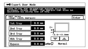
9 Check that the left margin of the test pattern for the second side is between 2.5 mm and 3.5 mm.
